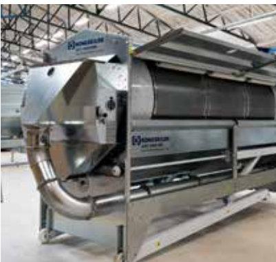
It is easy to open the side panels which saves time and increases efficiency when changing screens.
