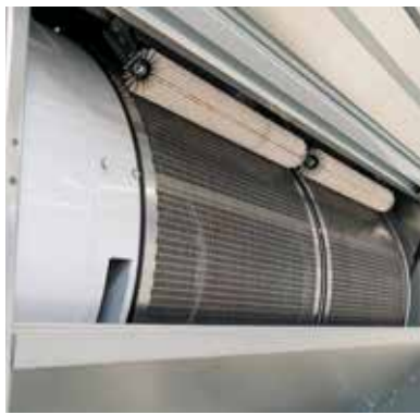
The cleaning brushes are mounted on a spring loaded arm for efficient even load on the outer screens.
