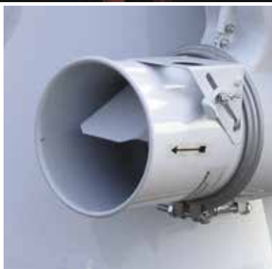
Air regulation for adjustment of the suction power of the aspirator.
