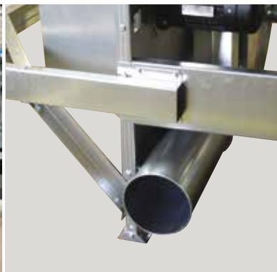
Screenings are conveyed through pipes up to 15 m away.
